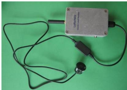
Option 1: Separate sensor and node
