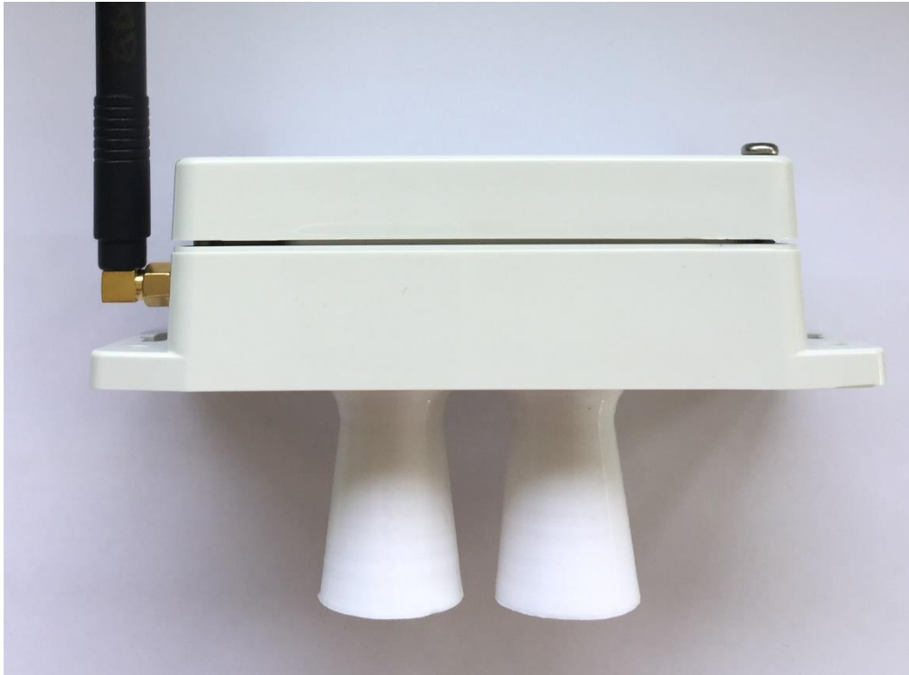
Standard Enclosure With Integrated Sensor and Communications Node
